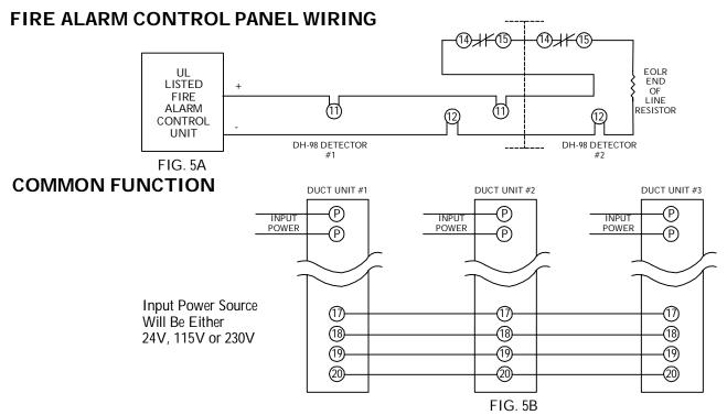
Installation requiring common functions must be wired as shown in Figure 5B.
