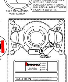
FIG. 6 MAGNET PLACEMENT
